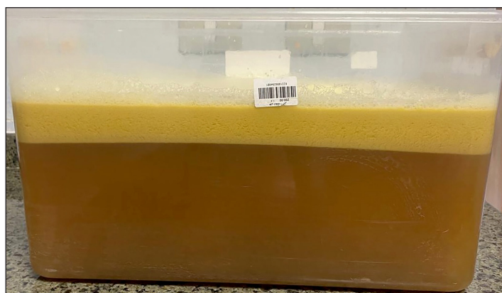
Figure 2. Separation of the soap from the sample
