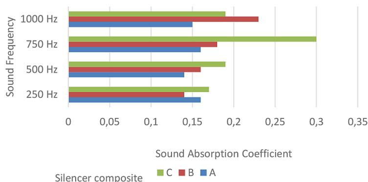
**Figure 2.** Sound absorption coefficient results of composite
