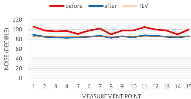
Figure 4. Noise intensity before and after using damper
