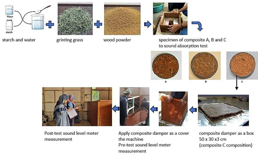
Figure 3. Measurement of noise intensity after used noise damper composite
