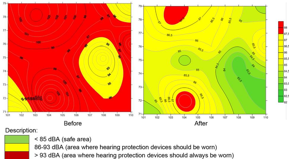
Figure 5. Noise mapping area before and after used damper
