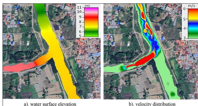
**Figure 6.** Water surface elevation and velocity distributions at river confluence
