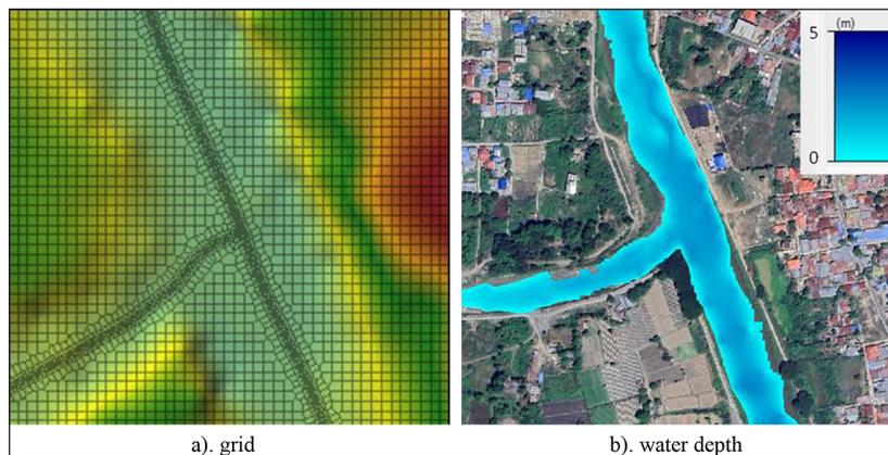
**Figure 5.** Domain grid and water surface elevations at river confluence
