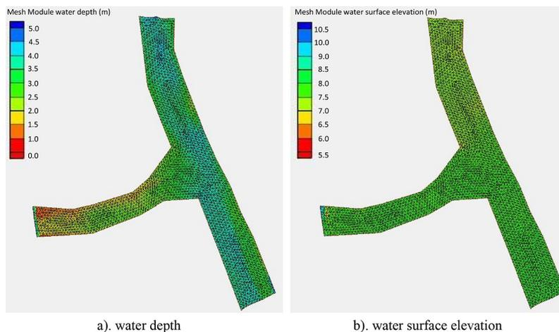
Figure 8. Water depth and water surface elevation
