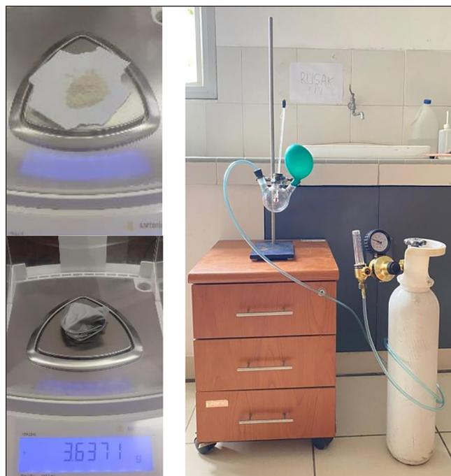
Figure 5. (a) Adsorbent and encapsulated within a balloon, (b) adsorption process experiment
