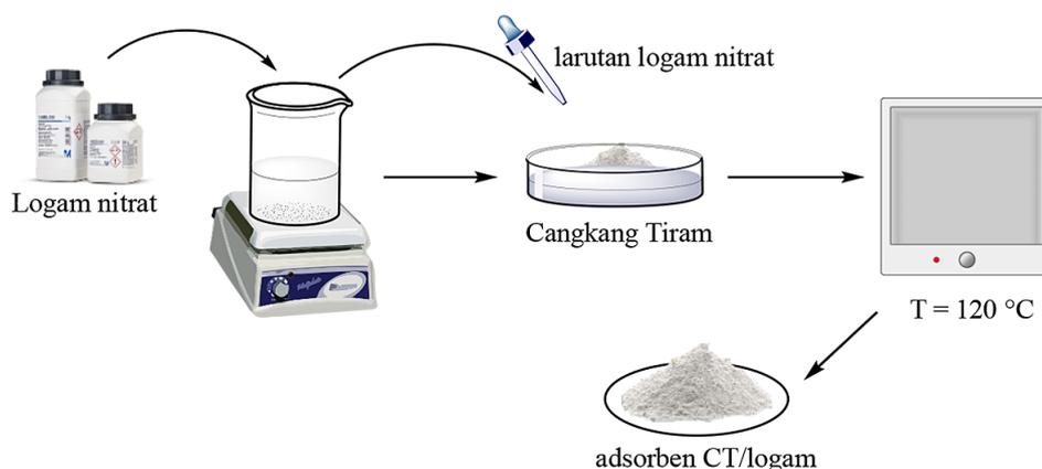
**Figure 1.** The schematic of the SIWI method used for adsorbent preparation
