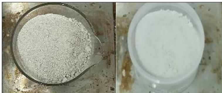
**Figure 3.** a) adsorbent OS/Al, b) adsorbent OS/Mg
