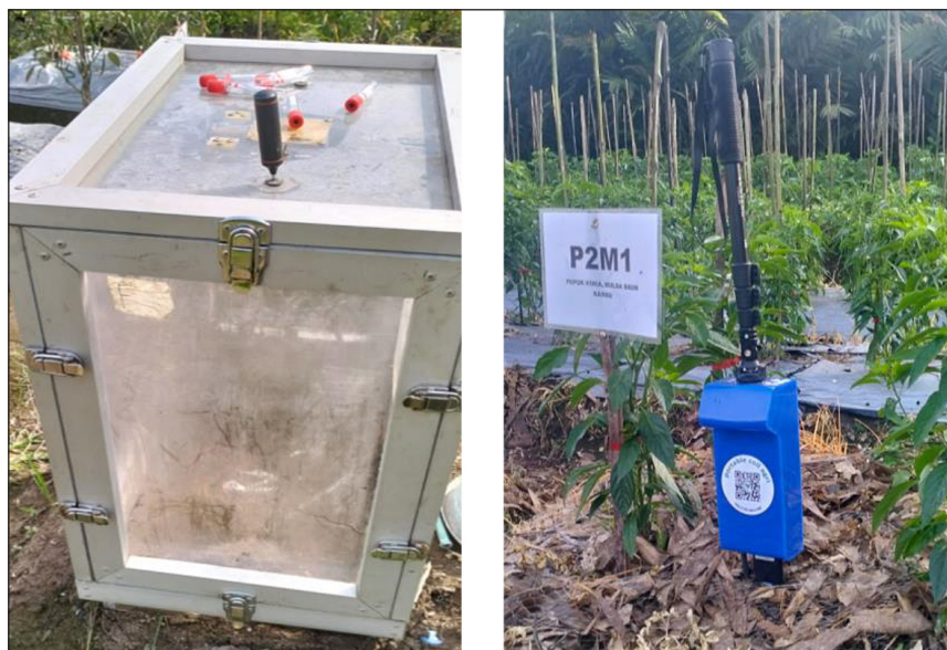
Figure 4. Closed chamber and soil monitoring system
