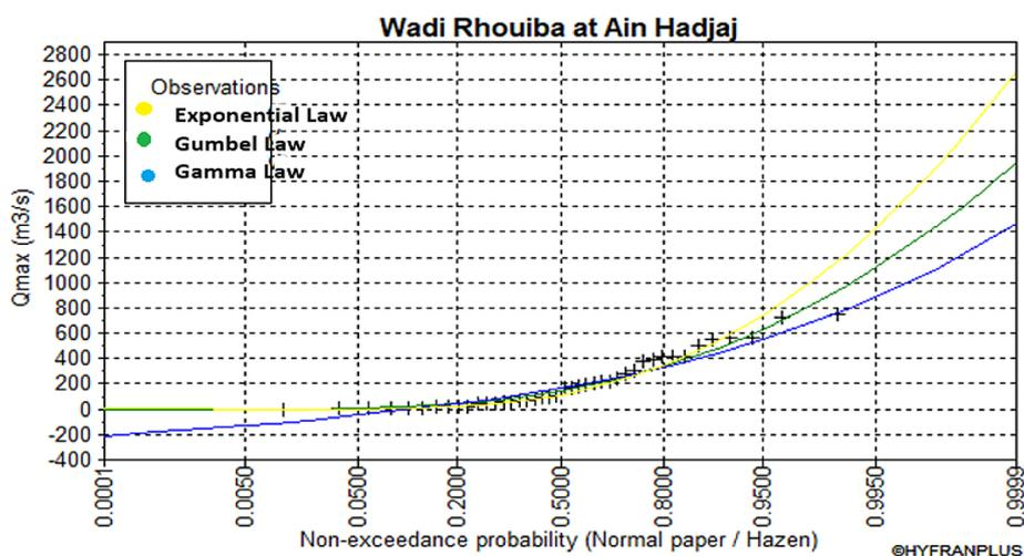
**Figure 11.** Adjustment of maximum flow rates to Gamma, Exponential and Gumbel laws
