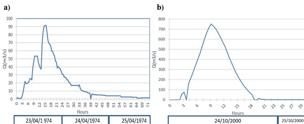
**Figure 10.** Example of a flood hydrograph for Wadi Rhouiba: a) the flood from 23/04/1974 to 25/04/1974; b) the flood from 24/10/2000 to 25/10/2000
