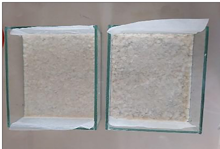
Figure 3. Membrane of cellulose corn stalks
