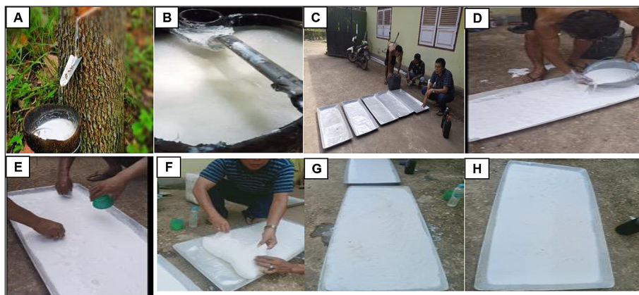
Figure 13. Collecting the latex (a-b), application of latex with liquid smoke (c-e), product of latex after added liquid smoke (f-h)
