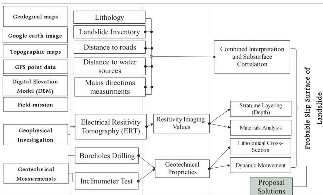
Figure 3. Methodology workflow for subsurface characterization of the landslide
