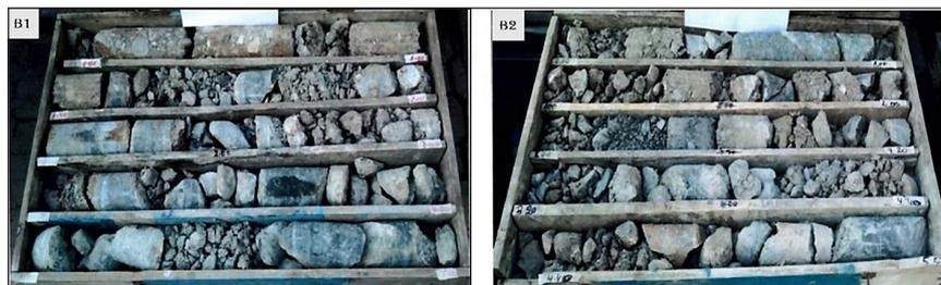
**Figure 4.** The first core sections from drillings B1 and B2 in depth 1 to 5 m
