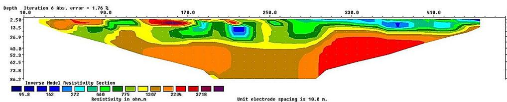
Figure 7. Longitudinal ERT profile implementation and resistivity model obtained
