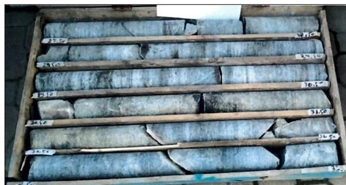
**Figure 5.** Core section from drilling B2 between 27.50 and 33.50 m
