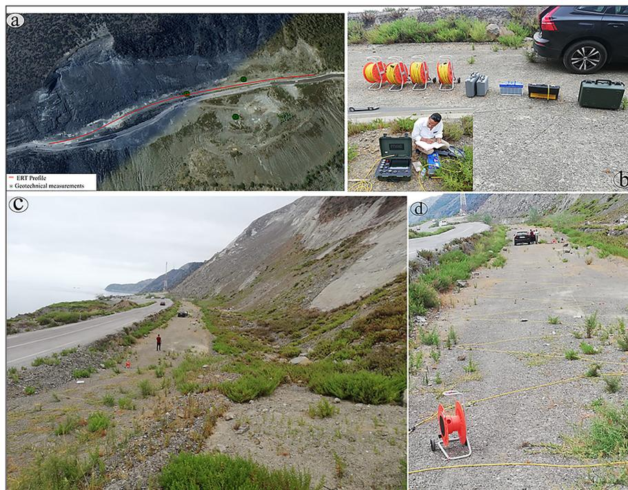
**Figure 2.** Site investigation for slope stability analysis: (a) geophysical and geotechnical measurement locations, (b) equipment for electrical resistivity tomography, (c-d) profile alignment along the slope using the Wenner-Schlumberger array
