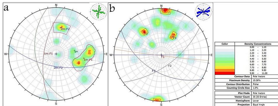
**Figure 10.** Fracture planes orientations at both the toe of the landslide and in areas beyond it
