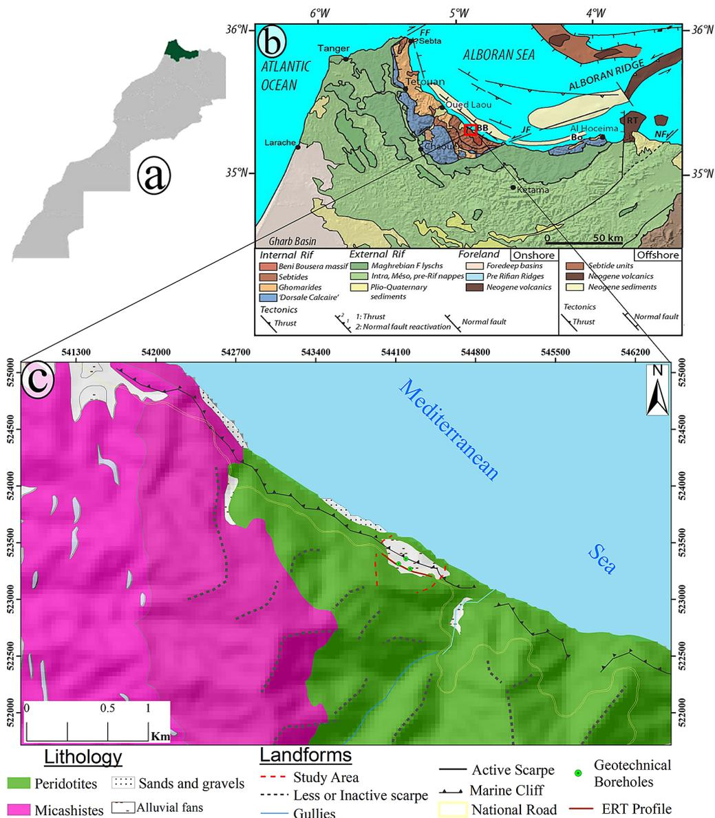
**Figure 1.** a) Morocco regions Map; b) Tectonic and geological framework of the Rif and southern Alboran Sea (Chalouan and Michard, 1990), c) Lithological and geomorphological maps of the studied landslide with geophysical and geotechnical measurements locations
