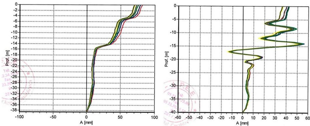
Figure 6. Deformation profile in drilling Borehole 2 (left) and in Borehole 3 (right)
