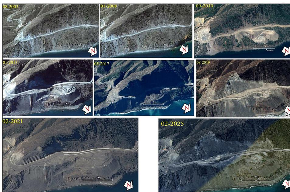
**Figure 8.** Monitoring the evolution of the studied landslide (2003–2025), using Google Earth Imagery
