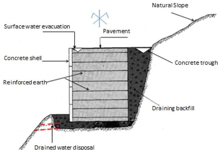
**Figure 11.** Proposal stabilization solution for the platform using the reinforced earth method
