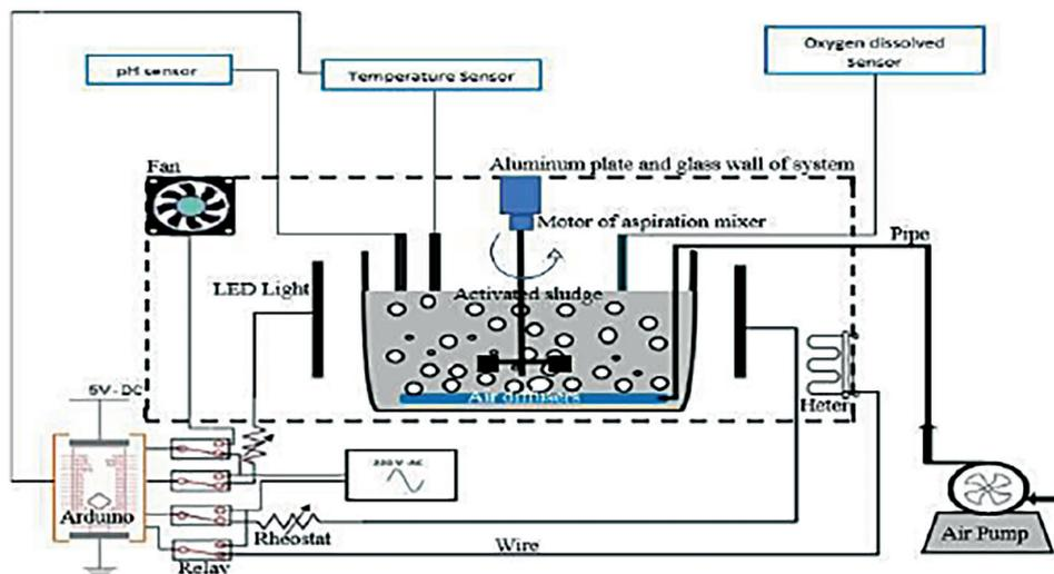
**Figure 1.** Schematic diagram of the experimental setup of activated sludge
