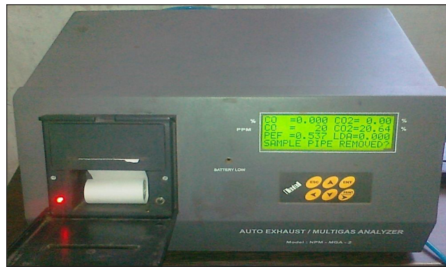
Figure 4. Multi gas analyzer for measuring the exhaust emissions concentrations
