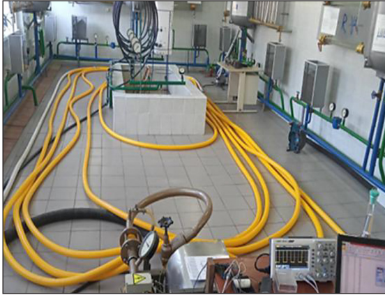
Figure 3. Photo of the hose line L = 140 m
