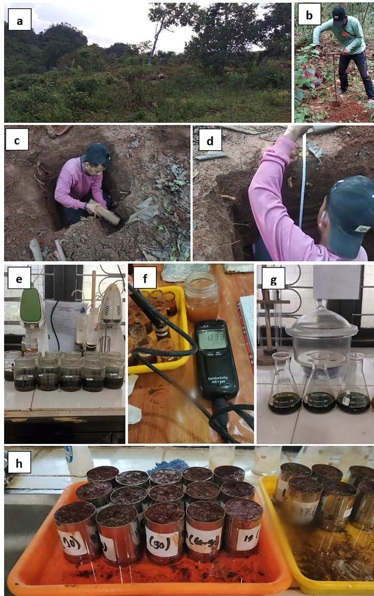
Figure 2. The research process involves several stages, beginning with field surveys at the initial stage, which include: a) Identifying the location for soil sampling in the Jompi watershed; b) collecting soil samples using a soil drill; c) employing the ring method for sample collection; d) measuring the depth of the soil; and proceeding to the laboratory analysis stage, which encompasses; e) analysis of soil texture; f) testing for soil salinity; g) analysis of soil C-organic; h) conducting soil permeability tests.
