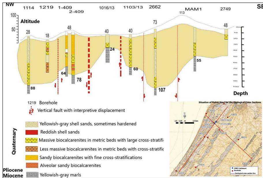
Figure 4. Geological cross-section in the Taïcha area perpendicular to the coast (ONEE, 2014)
