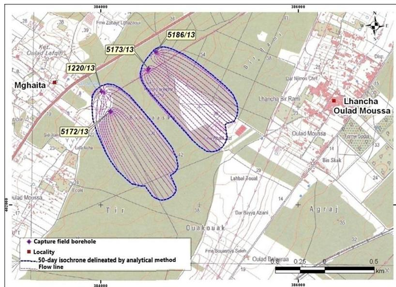
Figure 10. Delimitation of the 50-day isochrone using the analytical elements method
