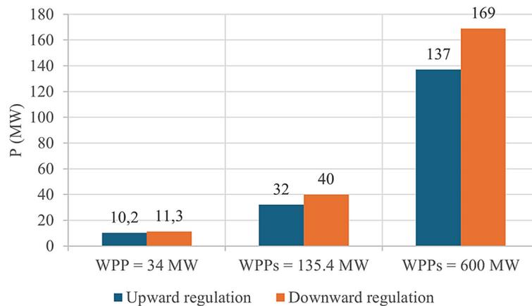
**Figure 13.** Required upward and downward regulation power as a function of total installed WPPs capacity in the Kosovo power system
