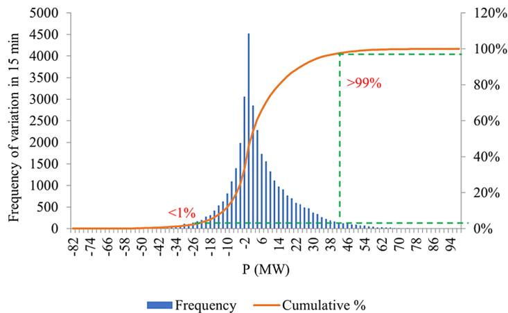
Figure 8. Total power imbalances of WPPs in the Kosovo power system as observed by the TSO
