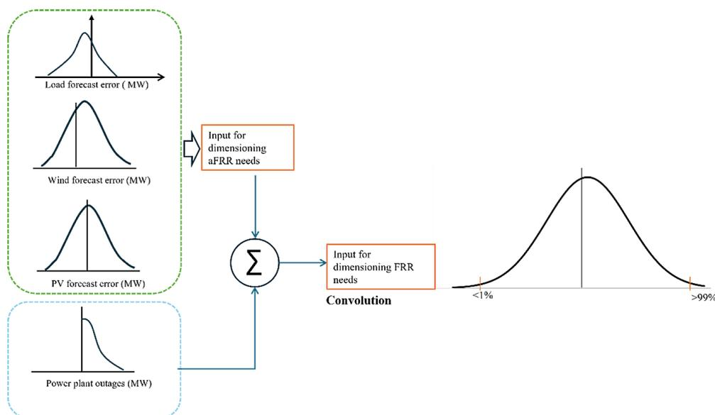
Figure 1. Probabilistic dimensioning of TSO balancing reserves [Hirth & Ziegenhagen, 2015]
