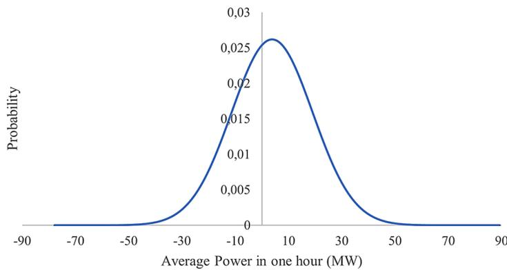
Figure 10. Normal distribution curve: 1-hour imbalance probabilities caused by WPPs in the Kosovo power system
