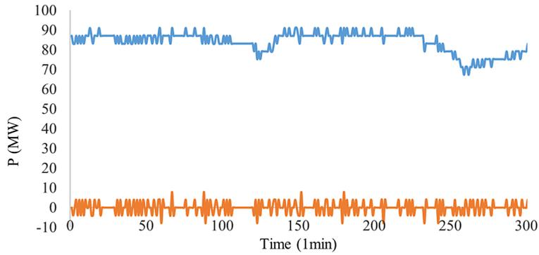
Figure 2. Average power variability of WPPs per minute of WPP Selaci (103.41 MW)
