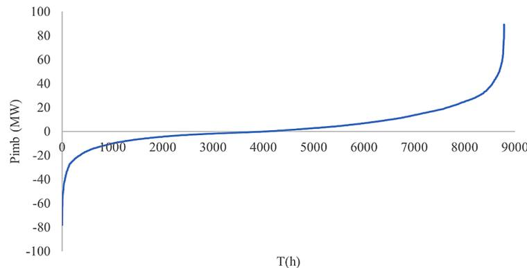
**Figure 12.** Imbalance duration Curve for WPPs in the Kosovo power system.
