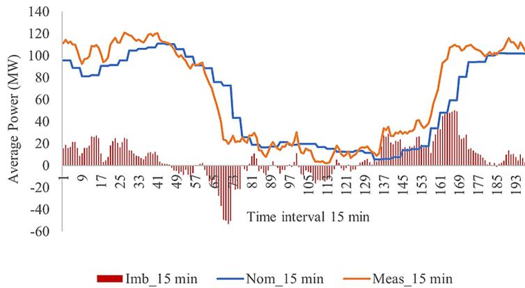
**Figure 11.** Comparison of 15-minute measured and forecasted wind power, along with the resulting imbalances in Kosovo's power
