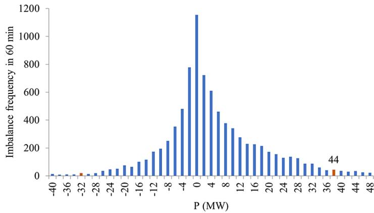
Figure 9. Histogram of imbalances caused by forecast errors of WPPs in Kosovo
