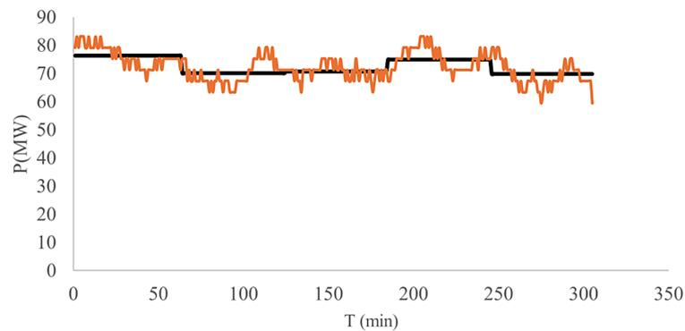
Figure 4. Average power over one hour and 1 min power variation of WPP
