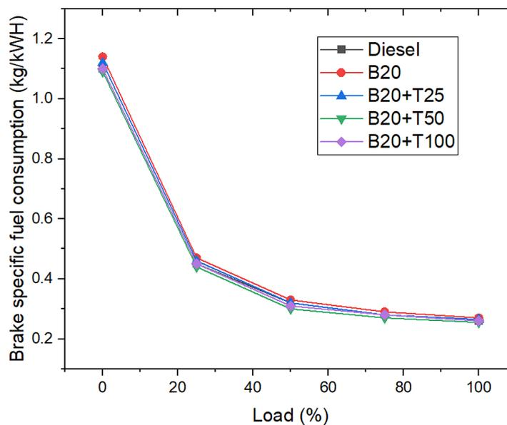
Figure 4. Brake specific fuel consumption with change in engine load
