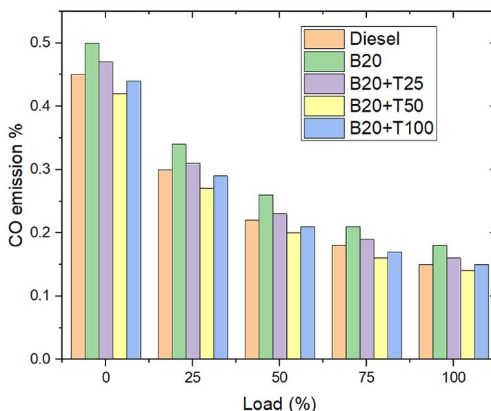
Figure 5. CO emissions with change in load
