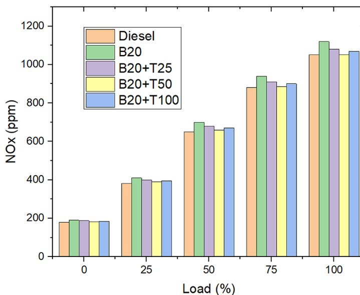
Figure 7. NO<sub>x</sub> emissions with change in engine load
