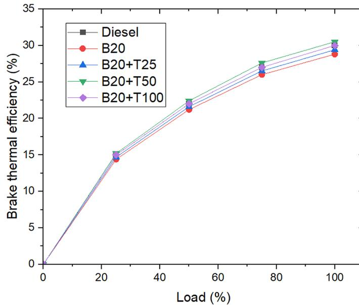
Figure 3. Brake thermal efficiency with change in engine load
