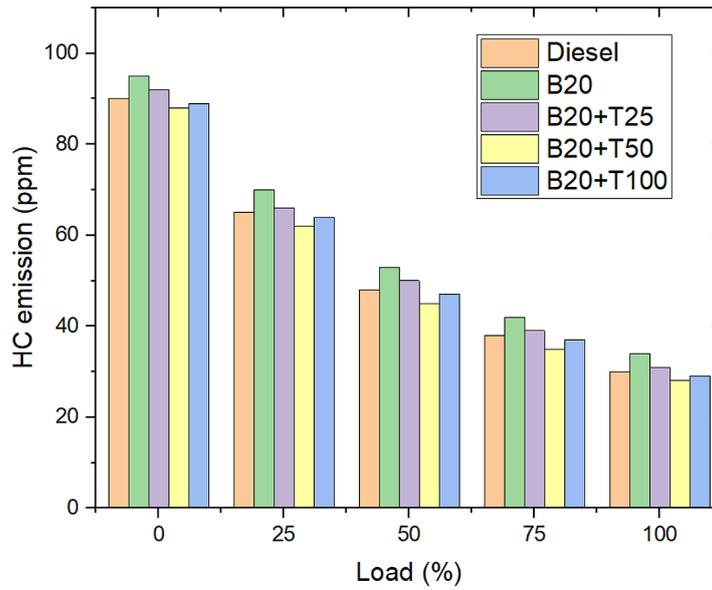
Figure 6. HC emissions with change in engine load
