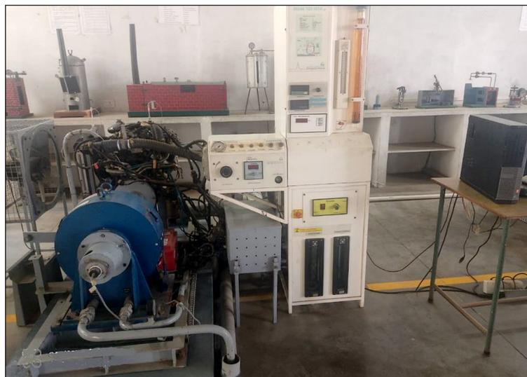
**Figure 1.** Pictorial representation of CRDI engine experimental test rig
