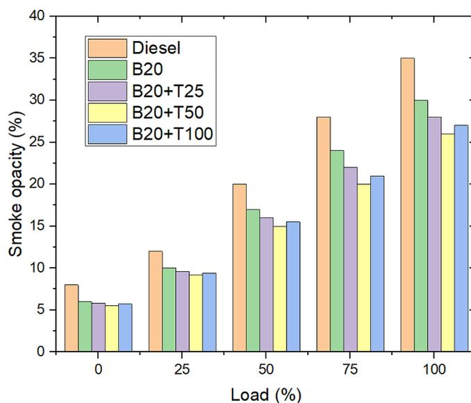
Figure 8. Smoke opacity with load variation
