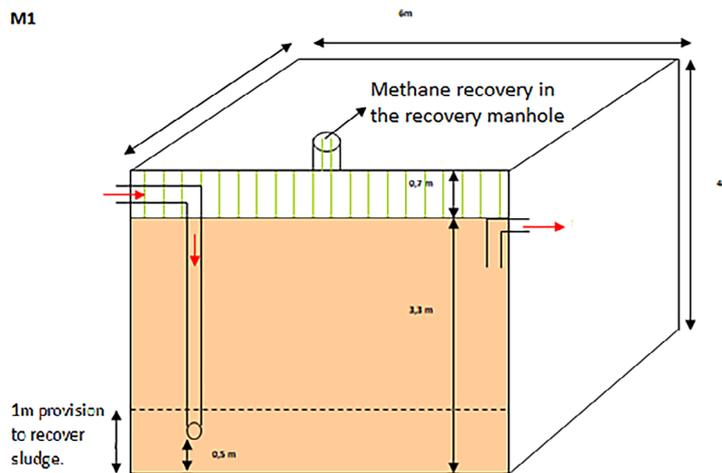
Figure 4. Design of methane production
