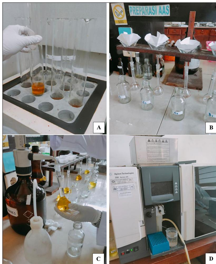
**Figure 4.** Laboratory procedures for heavy metal analysis, (A) soil digestion using a mixture of concentrated acids ( $\text{H}_2\text{SO}_4$ ,  $\text{H}_2\text{O}_2$ ,  $\text{HCl}$ ); (B) filtration of the digested solution using Whatman No. 42 filter paper; (C) dilution of the filtrate with deionized water to a final volume of 50 mL; (D) measurement of metal concentrations (Pb, Cd, Cu, Cr) using atomic absorption spectrophotometry (AAS)
