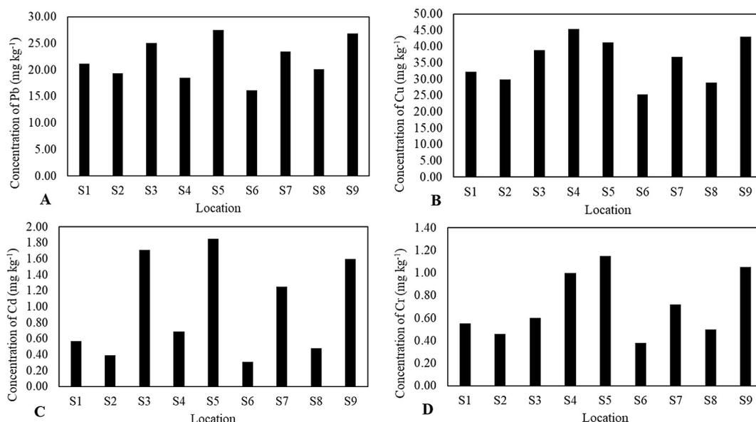
**Figure 5.** Spatial distribution of heavy metal concentrations in surface soils of Benoa Bay, Indonesia, where (A) Lead (Pb), (B) Copper (Cu), (C) Cadmium (Cd), and (D) Chromium (Cr), and Each bar represents the average concentration from a composite sample per location (S1–S9)
