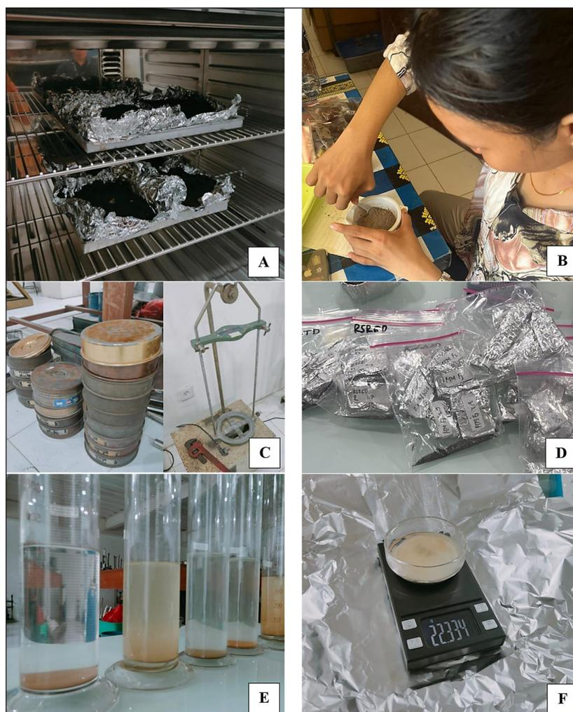
**Figure 3.** Laboratory procedures for soil particle size analysis, (A) oven-drying of soil samples at 60 °C, (B) gentle disaggregation using a ceramic mortar and pestle, (C) dry sieving of sand fractions using an ABM mechanical sieve shaker; (D) sieved soil fractions stored in aluminum foil, (E) pipette method for analyzing fine silt and clay fractions; (F) final weighing of oven-dried fine particles to determine soil type percentage
