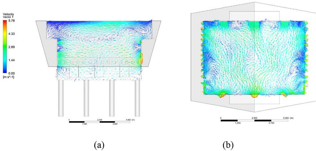
**Figure 14.** The airflow running throughout the Acehese traditional house simulated in Ansys: (a) vertical, (b) horizontal section at 12:00 local time (UTC+7)
