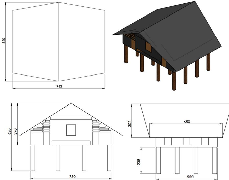
Figure 5. The dimension of the Acehnese traditional house model
