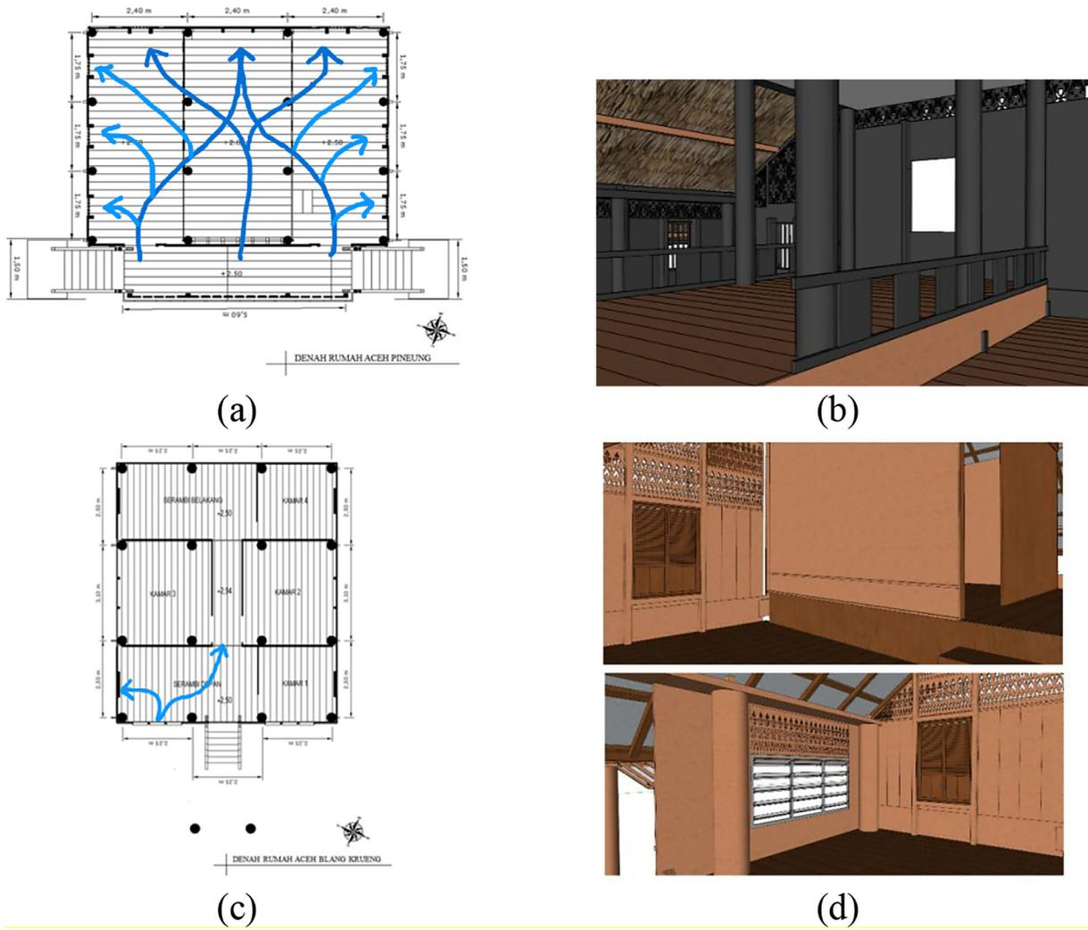
**Figure 12.** (a) airflow movement in House 1, (b) space conditions in House 1, (c) airflow movement in the space of House 2, (d) space conditions in House 2.
