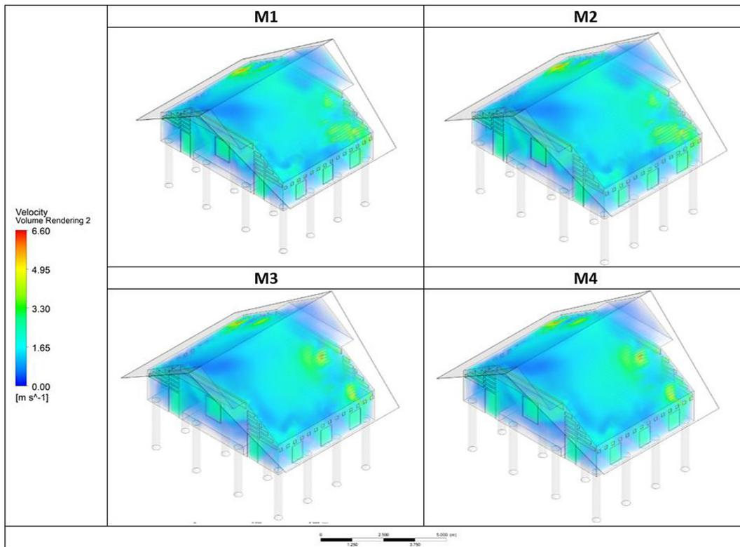
**Figure 15.** Air velocity simulation results of the four variations of Acehese traditional house at 12:00 local time (UTC+7)
