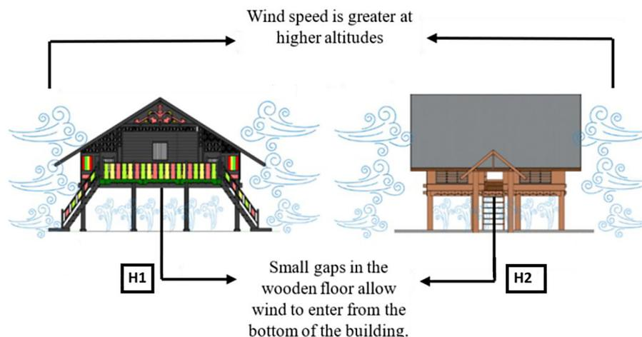
**Figure 10.** Effect of house height on thermal comfort for flowing the air
