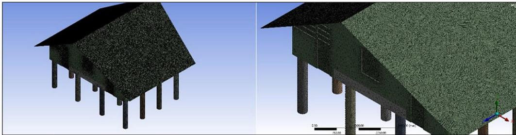
Figure 6. Meshing results in the research object
