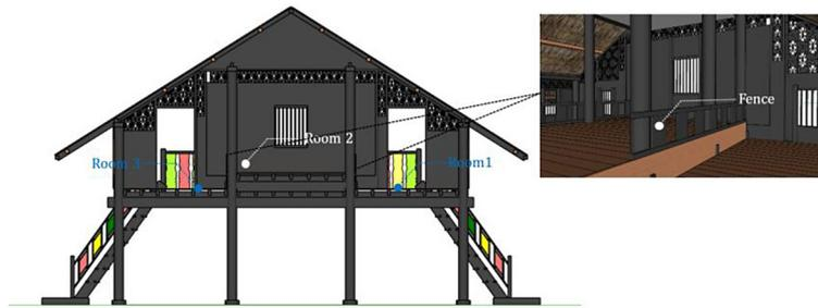
Figure 3. The split level distinguishing the space in House 1
