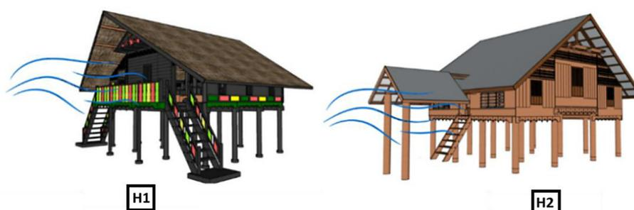
Figure 11. West wind entering a house that is oriented east-west
