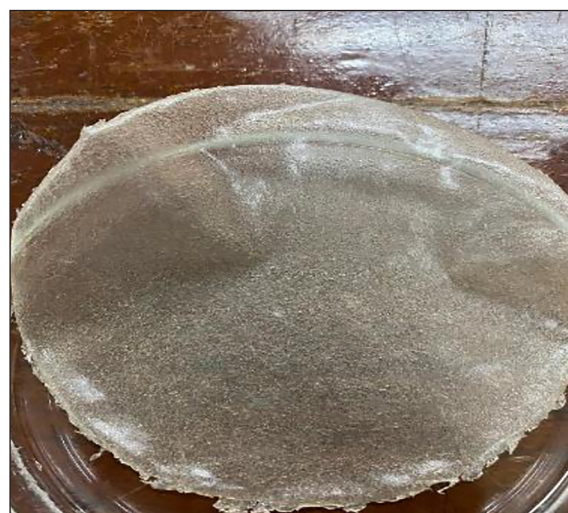
Figure 3. Edible film from cellulose of Eucheuma sp.
