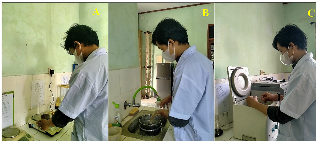
Figure 5. Weighing soil samples (A), filtering soil samples (B), and centrifuging of the soil filtrate (C)
