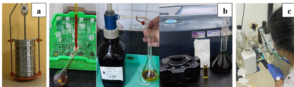
Figure 3. Analysis of sediment physicochemical parameters, (a) Grain size distribution, (b) C-organic content analysis using the Walkley and Black method, (c) Measurement of oxidation-reduction potential (ORP) and pH
