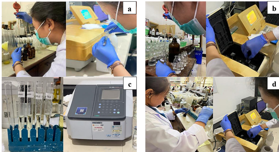
Figure 5. Laboratory procedures for inorganic nutrient analysis in sediment samples, with absorbance measured using a spectrophotometer at the respective wavelengths, (a) Ammonium ( \text{NH}_4^+ ), (b) Nitrite ( \text{NO}_2^- ), (c) Nitrate ( \text{NO}_3^- ), and (d) Phosphate ( \text{PO}_4^{3-} )
