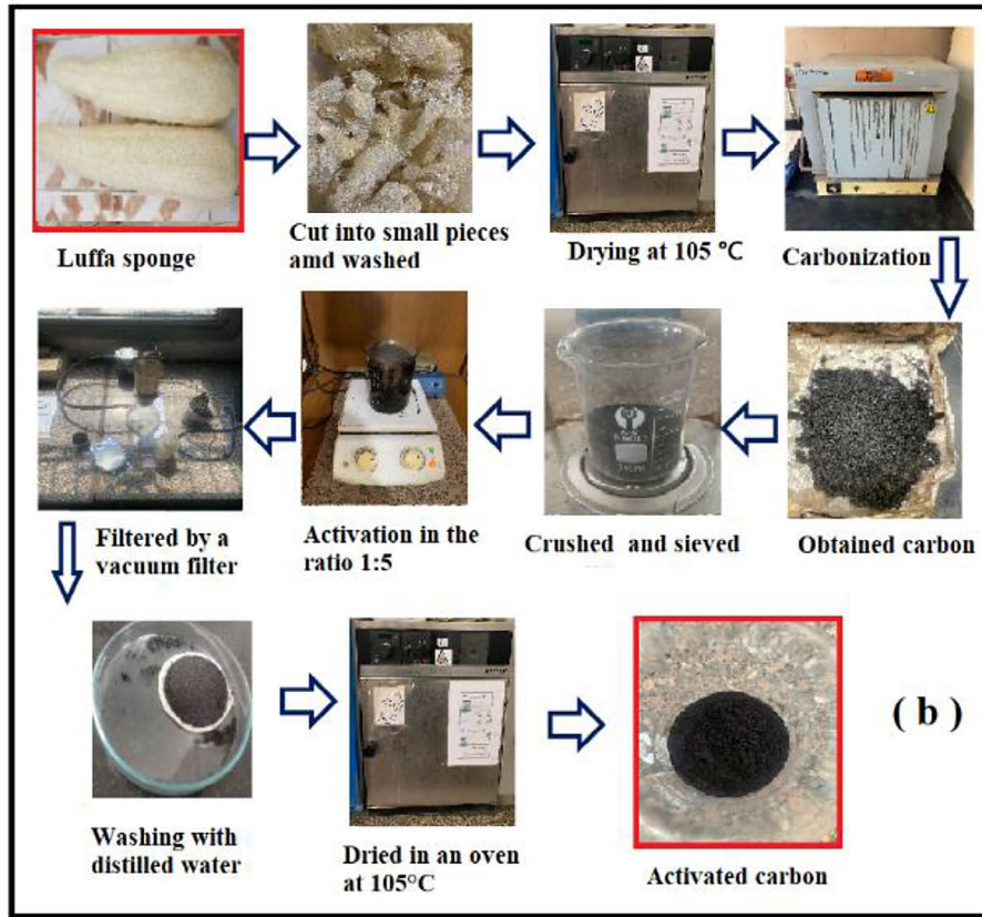
Figure 1. Cont. A schematic diagram of the experimental set up for the preparation of (a) CI-AC, (b) LU-AC and (c) CO-AC
