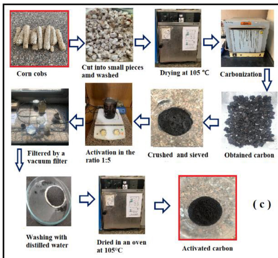
Figure 1. A schematic diagram of the experimental set up for the preparation of (a) CI-AC, (b) LU-AC and (c) CO-AC
