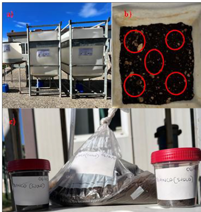
Figure 1. a) Pilot plant, b) sampling of soil in the tank, c) final sampler of soil
