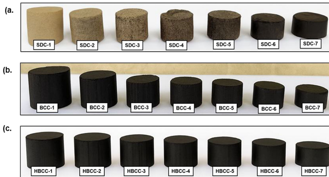
Figure 2. Physical characteristics of biomass–coal blending samples: (a) sago dregs–coal (SDC-1 to SDC-7), (b) biochar–coal (BCC-1 to BCC-7), (c) hybrid biocoke–coal (HBCC-1 to HBCC-7). The sample code variations indicate different blending ratios from 100% biomass (10:0) to 100% coal (0:10)
