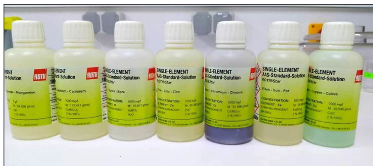
Figure 6. Atomic absorption spectroscopy-standards solutions for curve calibration
