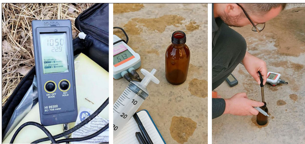
Figure 5. (a) Multiparameter HANNA HI 99300 for TDS and EC in filed measurement, (b) in field sample's filtration using 0.45\text{ }\mu\text{m} membrane filter, (c) sample acidification to pH of 1–2 by \text{HNO}_3
