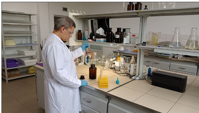
Figure 4. Addition of a chromic mixture (a mixture of potassium dichromate and sulfuric acid) to crushed, sieved, and weighed soil samples. Initial stage of soil analysis for organic matter determination
