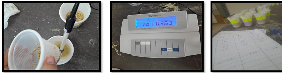
Figure 4. Measurement of the EC value of filtered water
