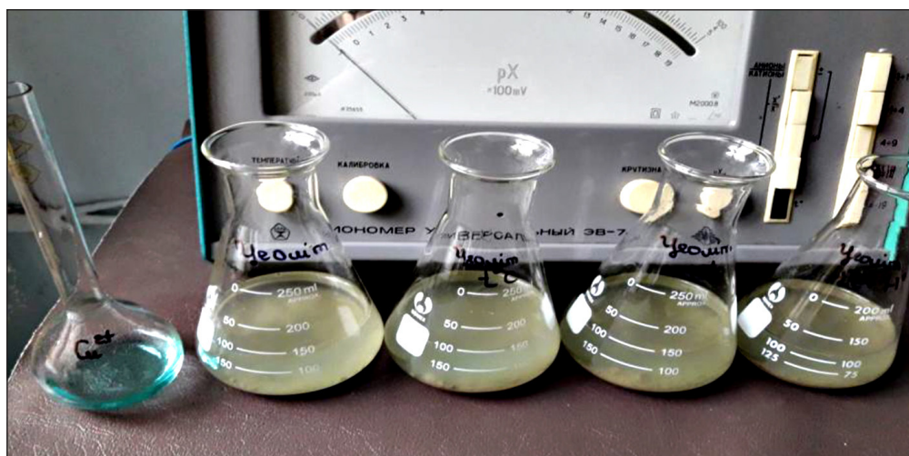
Figure 4. Contact time of the studied solutions required to establish adsorption equilibrium (illustrated by the zeolite– \text{Cu}^{2+} system; the initial model solution without sorbent is blue on the left)
