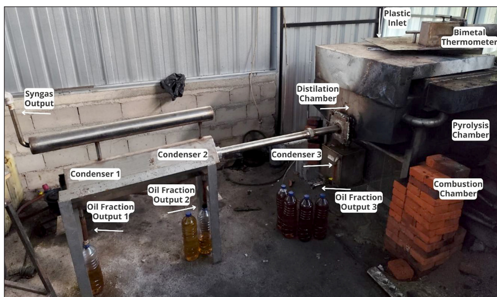
Figure 3. Integrated pyrolysis-distillation reactor configuration with three condensers mounted in series and parallel from the distillation chamber
