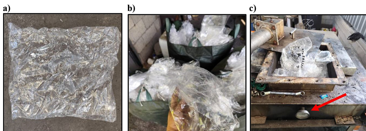
Figure 1. Condition of PP plastic waste (a) PP plastic whole form, (b) 10 kg PP plastic, (c) PP plastic in reactor and bimetal thermometer
