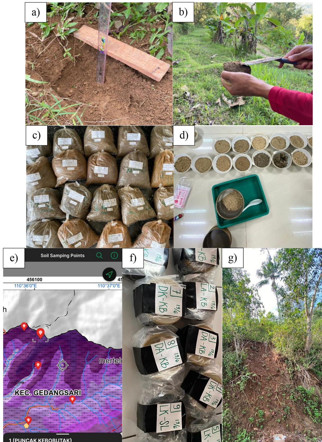
Figure 3. Field documentation and soil sample management: (a) mini pit preparation, (b) undisturbed soil samples were collected using a bulk density (BV) ring sampler, (c) disturbed soil sample collection and labeling, (d) air-dried soil samples prepared for laboratory testing, (e) soil sampling point locations displayed in Avenza Maps application, (f) undisturbed soil samples collected using bulk density rings, (g) field site conditions
