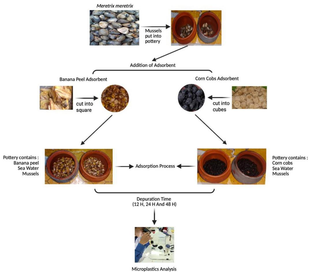
Figure 4. Illustration of the adsorbent production scheme and depuration process
