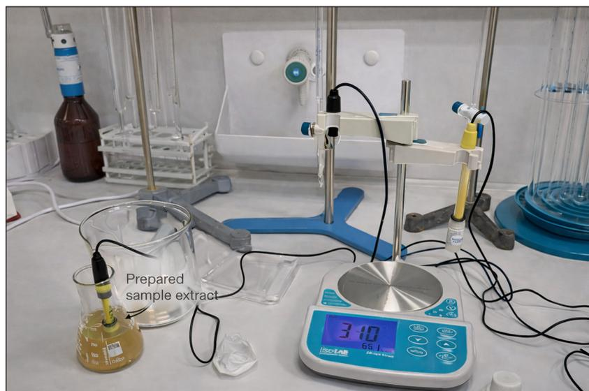
**Figure 2.** Multi-parameter analysis: pH, TDS, and electrical conductivity. The yellow liquid in the flask represents the aqueous extract of the dietary supplement sample used for measurement
