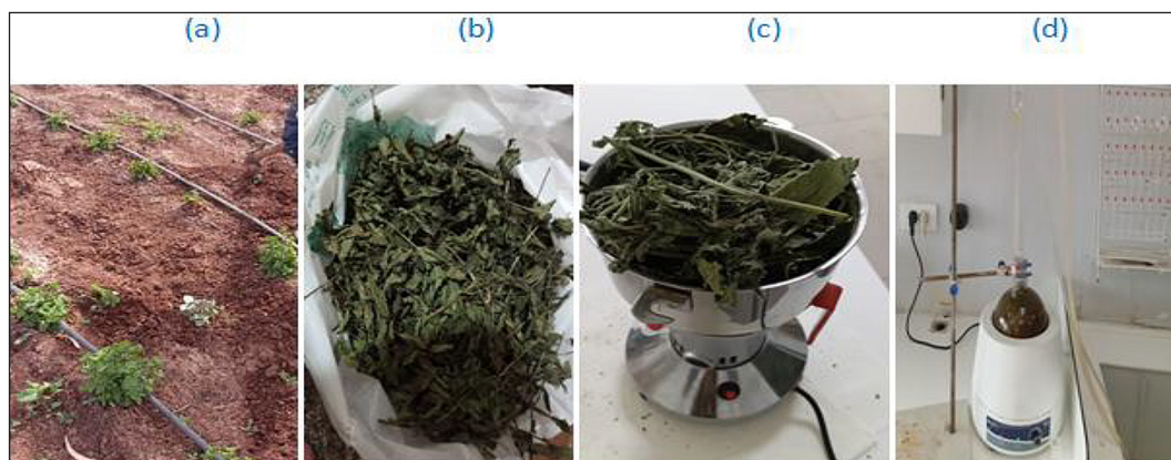
Figure 2. Sample preparation for analysis: (a) plant implantation, (b) dried plant, (c) plant shredder, (d) essential oil extraction
