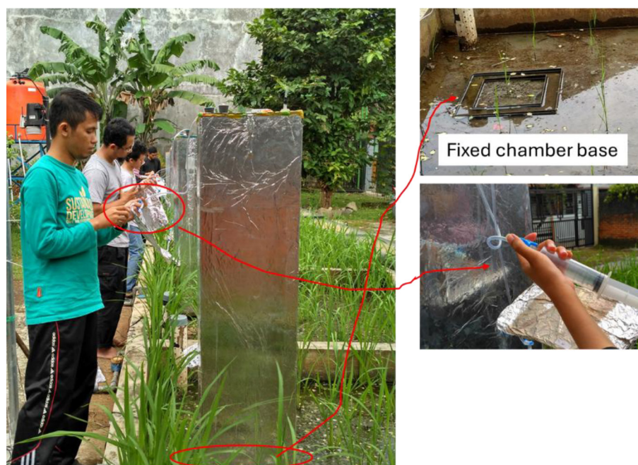
Figure 3. In situ greenhouse gas sampling using the closed static chamber method in experimental paddy plots
