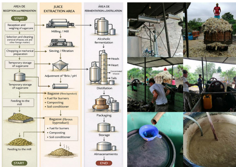
Figure 6. Production process of brandy from sugarcane ( Saccharum officinarum ) in small and medium-sized enterprises
