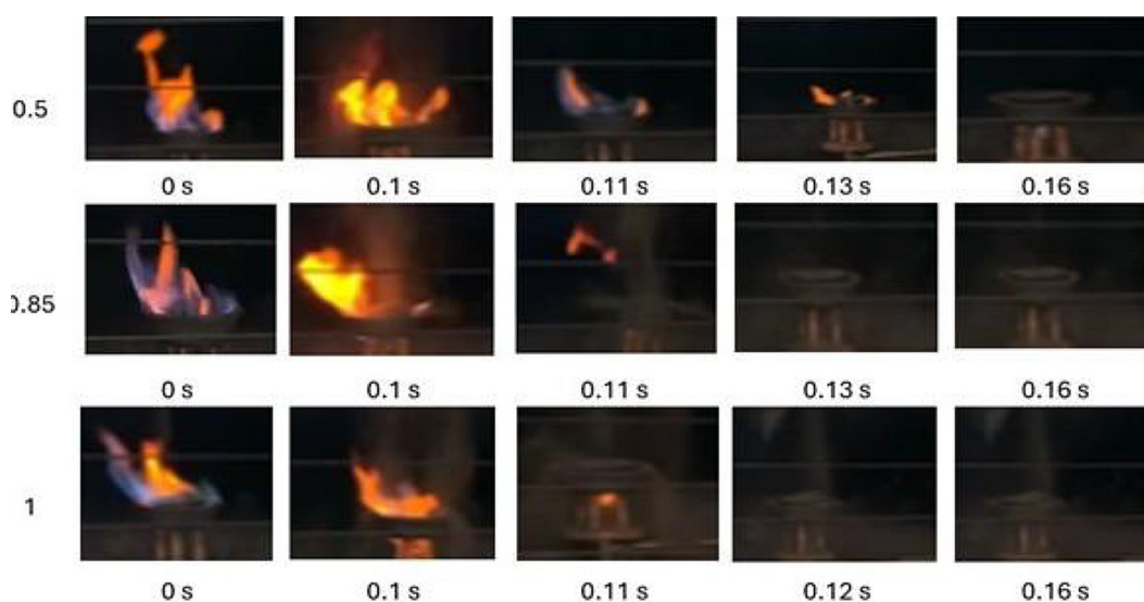
Figure 7. The process of extinguishing fire using Sidoarjo mud powder with the addition of 20% \text{SiO}_2
