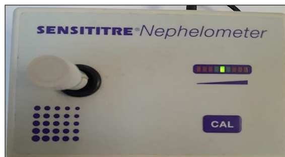
Figure 6. Nephelometer used for McFarland standard adjustment
