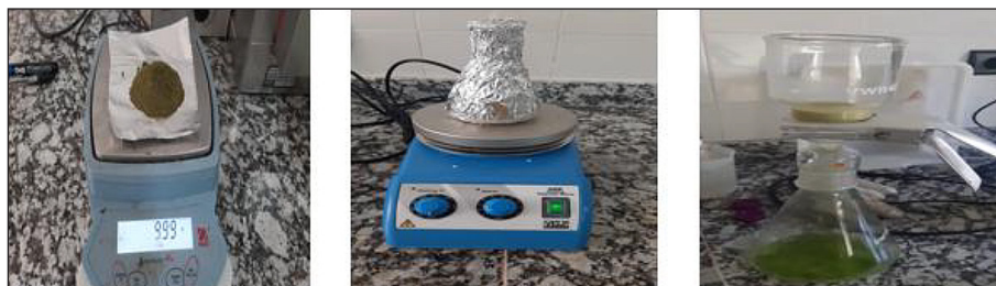
Figure 1. Maceration of Cannabis sativa L. leaf by-product powder in 70% ethanol under magnetic stirring
