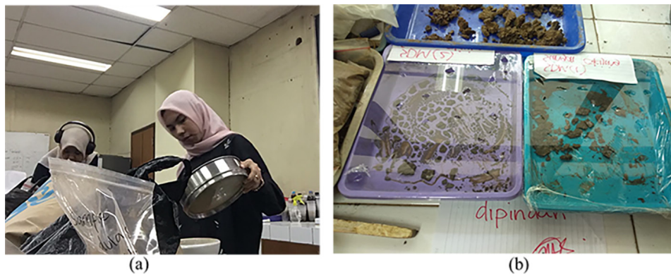
Figure 6. Laboratory preparation of sediment samples: (a) sieving using a 120-mesh sieve and (b) drying process prior to analysis
