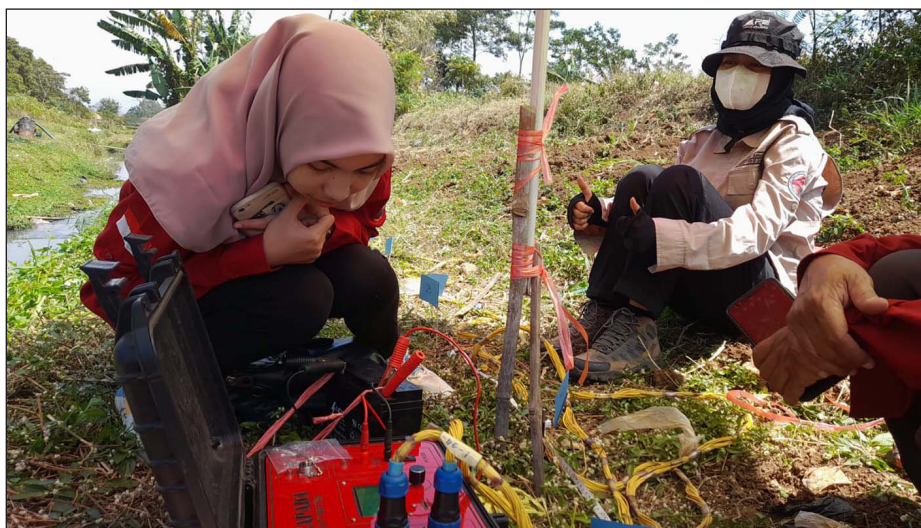
Figure 3. Data acquisition procedure using the RMSS Marcapada resistivity meter
