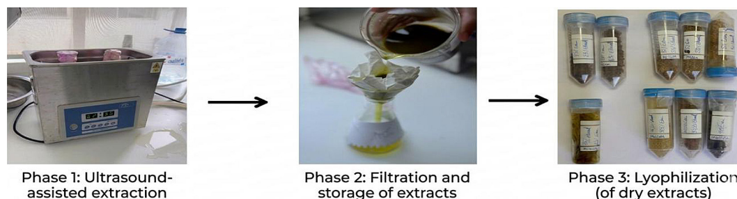
Figure 2. Sequential stages of the phytochemical extraction process, from ultrasound-assisted extraction to final lyophilization of dry botanical extracts
