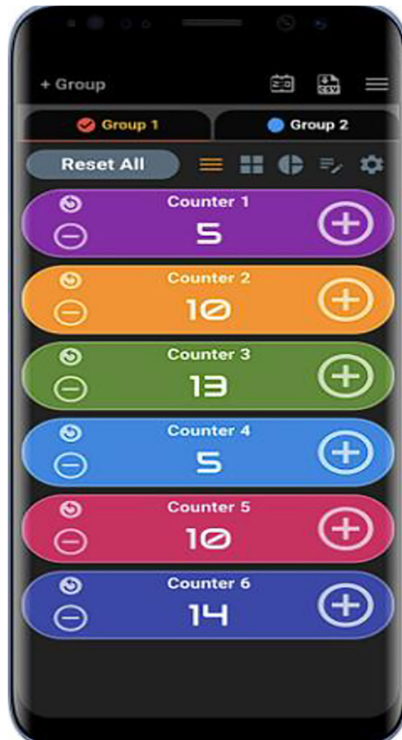
Figure 3. Android-based digital multi-counter application used for traffic volume survey at the Mandai Five-Leg intersection
