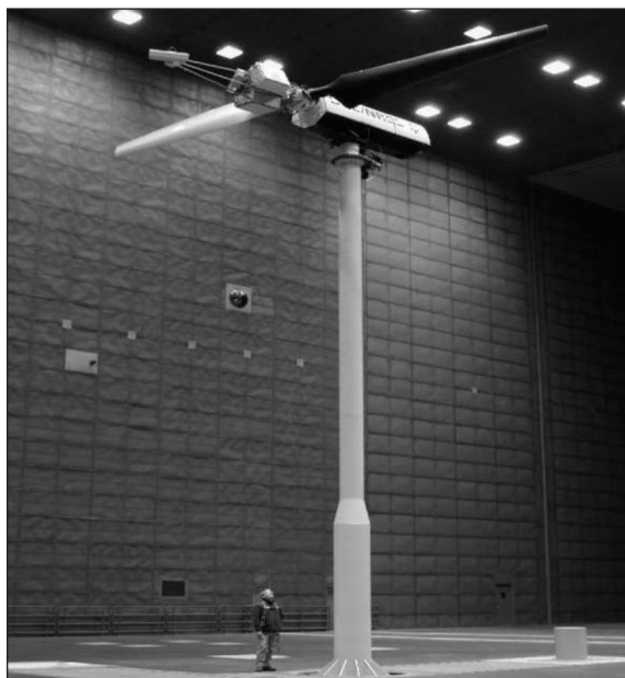
Figure 6. The NREL phase VI upwind turbine (Hand, 2001)
