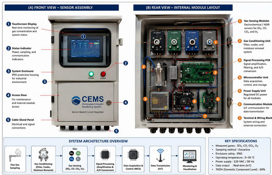
Figure 3. Integrated hardware architecture, calibration activities, and real operational deployment of the developed locally integrated sensor-based CEMS
