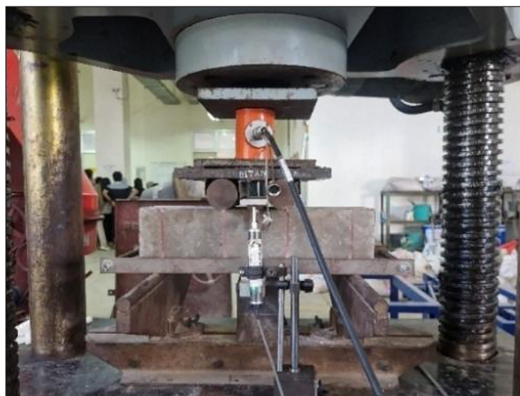
Figure 1. Setup for flexural strength test of concrete
