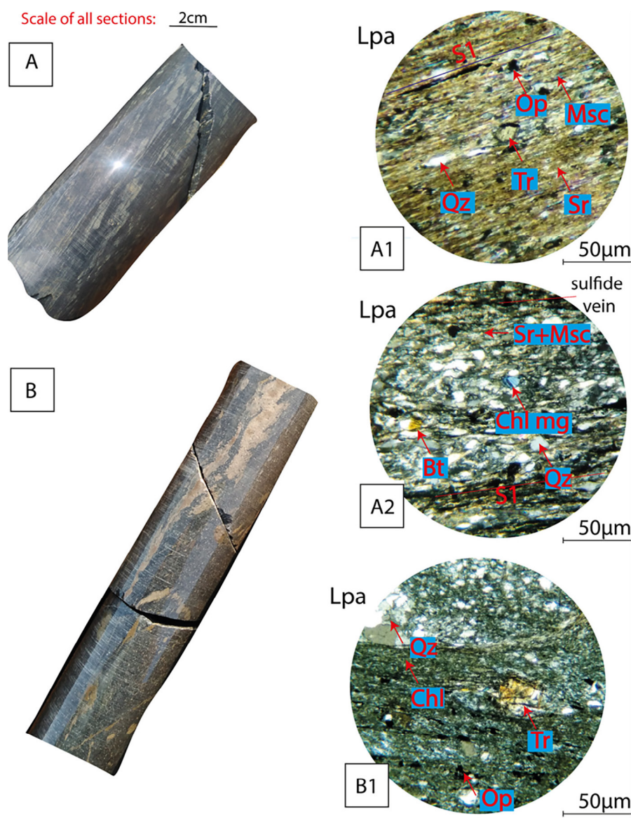
Figure 9. A) Macroscopic aspect of the hanging wall pelites; A1 and A2) Photomicrograph of hanging wall pelites (LP); B) Macroscopic aspect of the footwall sandy pelites; B1) Photomicrograph of the footwall sandy pelites (LP). Abbreviations: Qz: quartz; Mus: muscovite; Tor: tourmaline; Chl mg: magnesian chlorite; Op: opaque minerals; Ser: sericite; LP: crossed polarized light
