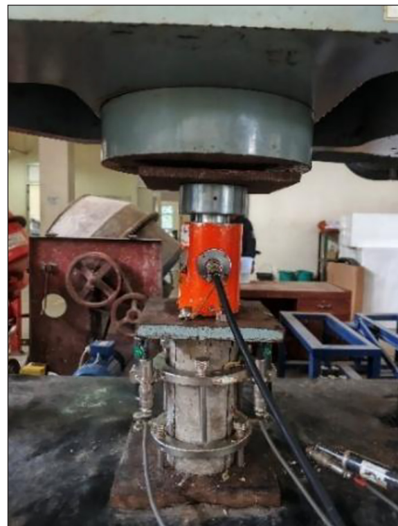
Figure 3. Compressive-strength test setup on the universal testing machine (UTM)
