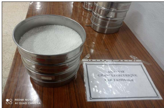
Figure 3. Granulometric analysis of the fertilizer by sieving. Photograph of the sieve stack used to separate the fertilizer into different particle-size classes before the spreading experiments
