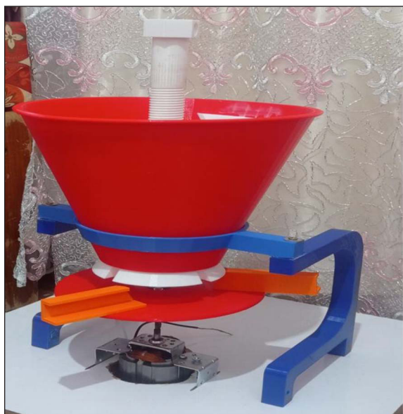
Figure 1. Quarter-scale centrifugal fertilizer spreading prototype fabricated at the Department of Mechanical and Agro-Industrial Engineering, Higher School of Engineers of Medjez El Bab. General view showing the hopper, supporting frame, motorized rotating disc, and experimental mounting system used during the indoor spreading tests
