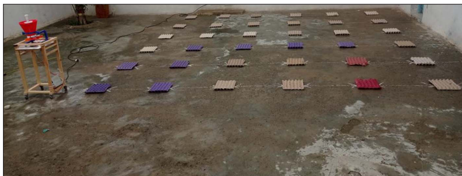
Figure 5. Experimental spreading layout. Indoor experimental setup showing the centrifugal spreader and the reception area used to collect and quantify the transverse distribution of fertilizer particles
