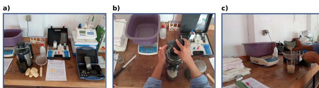
Figure 3. (a) Juice extraction equipment (centrifuge, fine-mesh membrane, Gluco-LIS), (b) potato juice extraction, (c) juice filtration using a fine-mesh membrane
