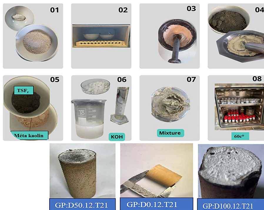
Figure 2. Flowchart of geopolymer preparation: (1) raw materials; (2) MK calcination at 750 °C for 5 h; (3–4) grinding; (5) sieved raw materials; (6) KOH solution preparation; (7) mixing; (8) curing. Lower images illustrate examples of synthesized geopolymer cylinders
